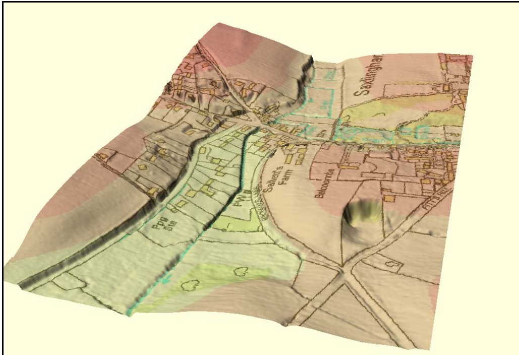
Figure 17: 3D representation of DTM with OS as presented in InfoWorks RS
